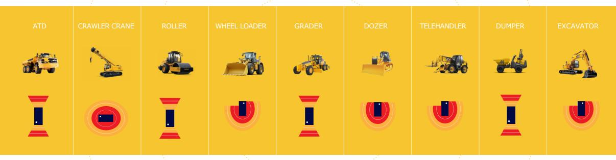
Examples of detection zone configurations. Zone configurations can be adapted depending on the requirements for each machine and site requirements.
